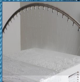
Rain Test Equipment
